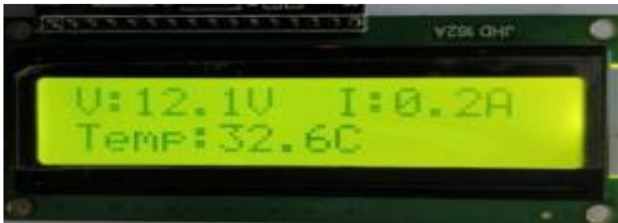
Figure 2 Display of Voltage, Current and Temperature
