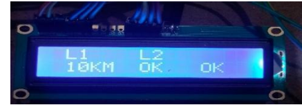
Figure 3.2 Fault Detection in Line
