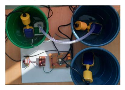
Automated water flow Control System in Overhead Tanks using Internet of Things and Mobile Application uses reliable sensors and mobile application. The application is being developed after testing various sensors and finding the best basing on the cost and work efficiency.
