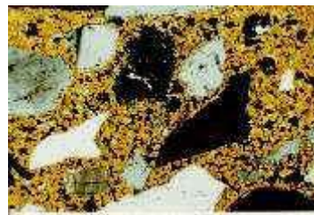
"Pop-corn" like calcite crystals present in carbonated paste. The concrete is suffering from bi-carbonation.
