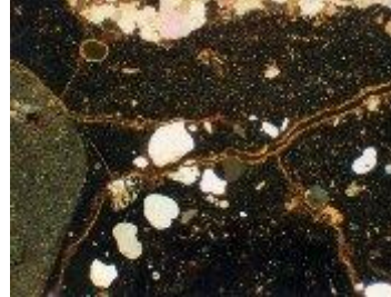
Carbonated paste along cracks inside a concrete. The cracks are formed due to alkali silica reaction.
