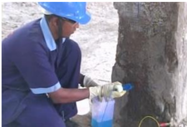
Half-Cell Potential Test of Column
