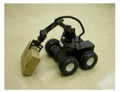
Robots are indispensable in many manufacturing industries. The reason is that the cost per hour to operate a robot is a fraction of the cost of the human labor needed to perform the same function. So in order to reduce human effort Pick and Carry robot is used, once it is programmed, it is repeatedly performed functions with a high accuracy that surpasses that of the most experienced human operator.
