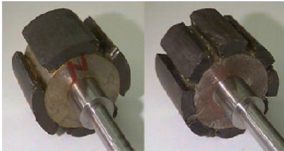
Fig. 3.2 Four pole and eight pole rotor of BLDC motor
