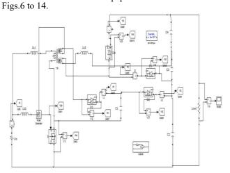
Fig.6.Matlab/simulation model of high step up Converter.
