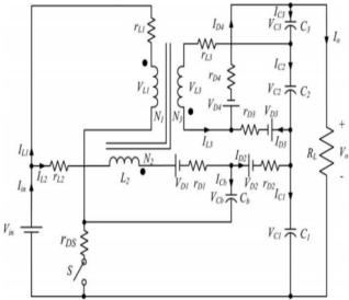
Fig. 5. Equivalent circuit including inductor conduction losses.
