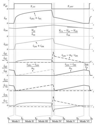
Fig. 3. Steady-state waveforms in CCM operation.
