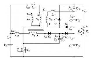
Fig. 2. Equivalent circuit of the proposed converter.
