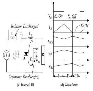
Fig.4. Operation of Cuk converter in DICM (Li) during (a-c) different Intervals of switching period and (d) the associated waveforms
