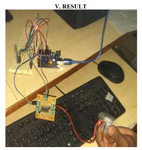
FIG: MOTOR turned ON through Voice command
