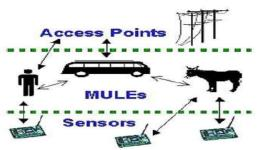
Fig2. The three tiers of the MULE architecture
