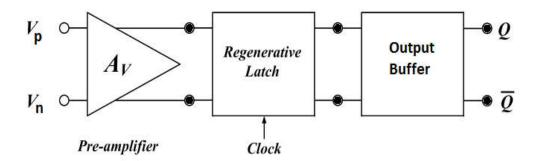
Fig: Block diagram of Comparator
