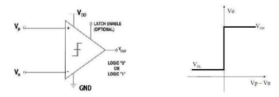
Fig: Schematic of Comparator
