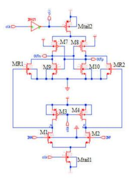
Fig 2: Schematic circuit of Conventional double tail dynamic comparator
