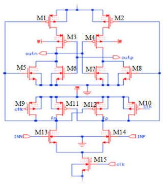
Fig 5: Schematic circuit of proposed comparator
