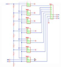
Fig 9: Schematic circuit of 3-Bit Flash ADC with proposed comparator
