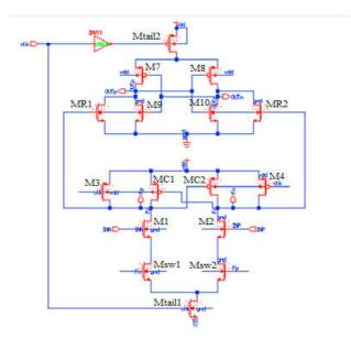
Figure 4: Schematic Circuit of Modified Double Tail Comparator b)Final Structure
