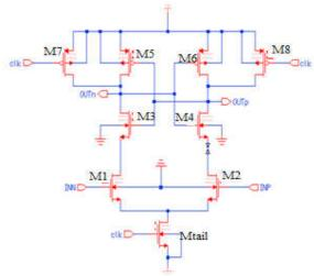
Fig 1: Schematic Circuit of Conventional dynamic comparator
