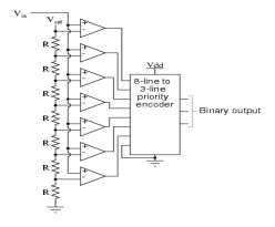
Fig 7: 3-Bit Flash ADC
