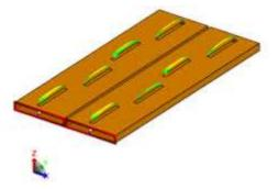
Fig. 1: Slotted Rectangular waveguide
