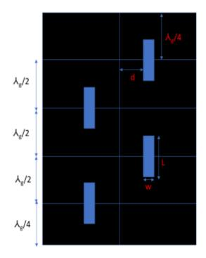
Fig. 2: Slotted Waveguide Antenna with 4 slots
