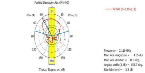
Fig.5:Radiation pattern of a Rectangular Slotted Waveguide Antenna
