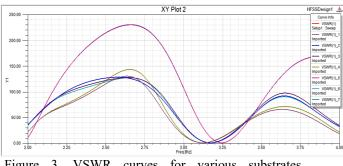
Figure 3. VSWR curves for various substrates materials.
