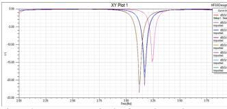
Figure 2. Return Loss in dB for various substrate materials.
