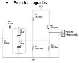
FIG 6:circuit diagram of repeller
