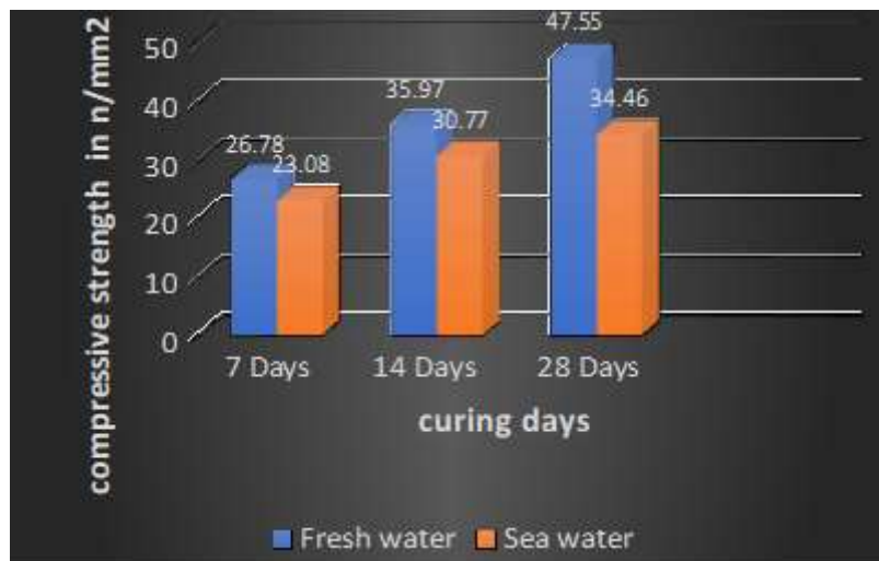
Compressive strength variation b/w Fresh water and Sea water
