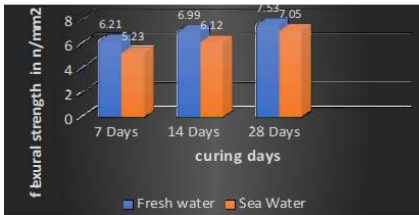
Flexural strength variation b/w Fresh water and Sea water
