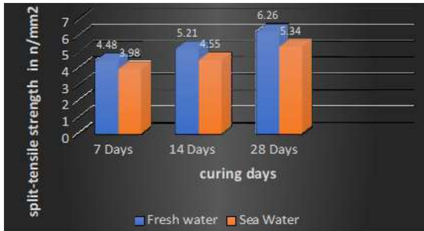
Split-Tensile strength variation b/w Fresh water and Sea water
