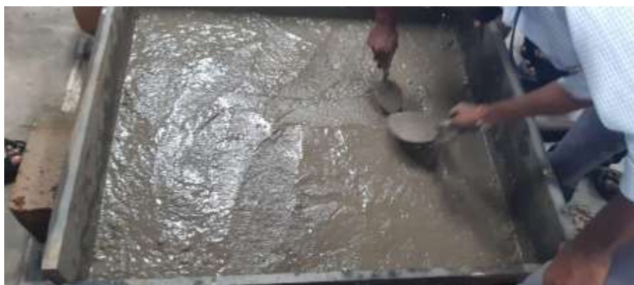
Fig.3.8.Polypropylene reinforced concrete slab
