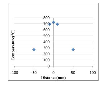
Fig 5.34 Temperature acting on the centre line of the specimen
