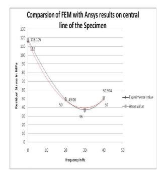
Fig 5.33 Comparison of FEM with Ansys results on central line of the Specimen
