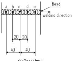
(b) On the bead Fig 3.1 Measuring locations of residual stress (mm)
