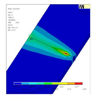
Fig.2 TEMPERATURE DISTRIBUTION AFTER WELDING
