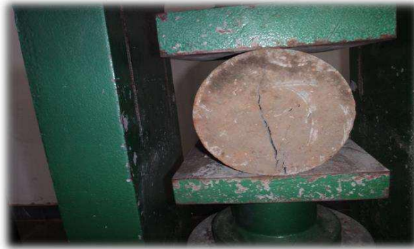
Fig.5.5.Split tensile strength testing of specimen
