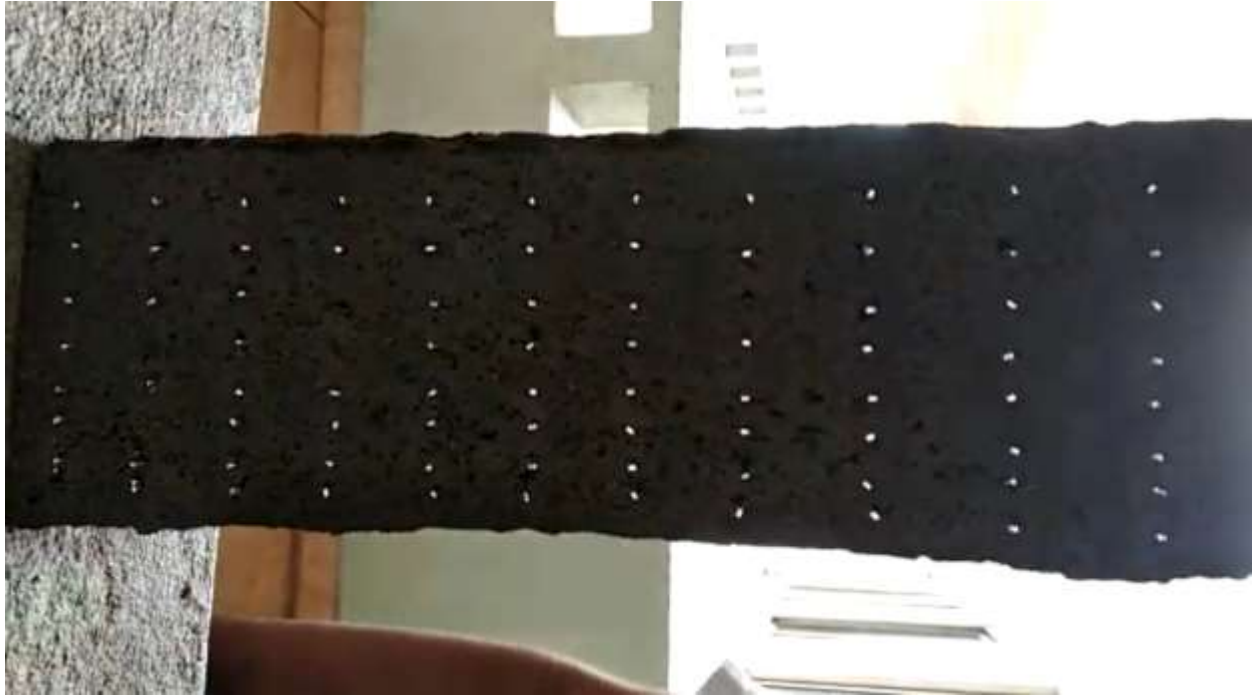
Light Transmitting Through Mortar Brick (Prototype Model)
