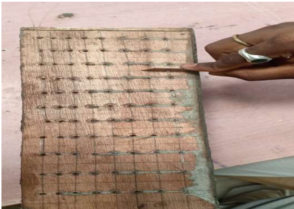
Inserting of optical Fibres into Prototype Model followed by Casting and Furnishing the Specimen
