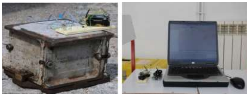
Figure 2 Continuous wireless temperature monitoring within a concrete cube. [55]
