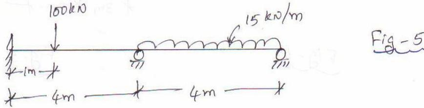
2. Analyse the beam shown in the Fig.5, using stiffness method
