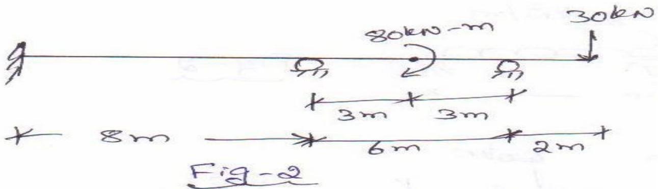
3. Analyse the frame shown in the Fig.2, by moment distribution method. Draw SFD & BMD
