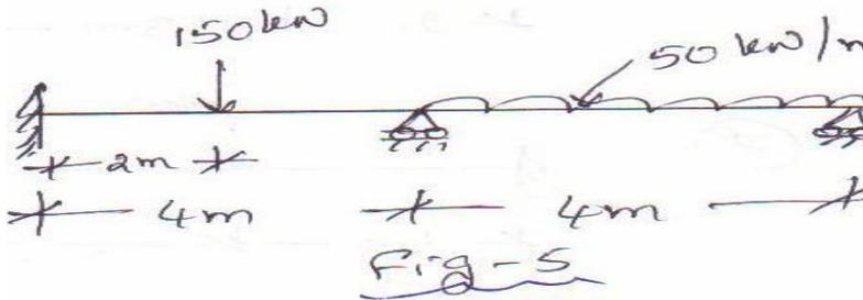
4. Analyse the beam shown in the Fig.5, using stiffness method
