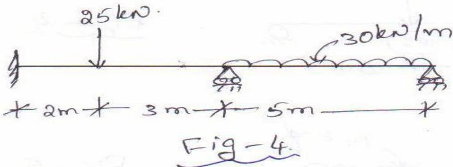
3. Analyse the beam shown in the Fig.4 using flexibility method
