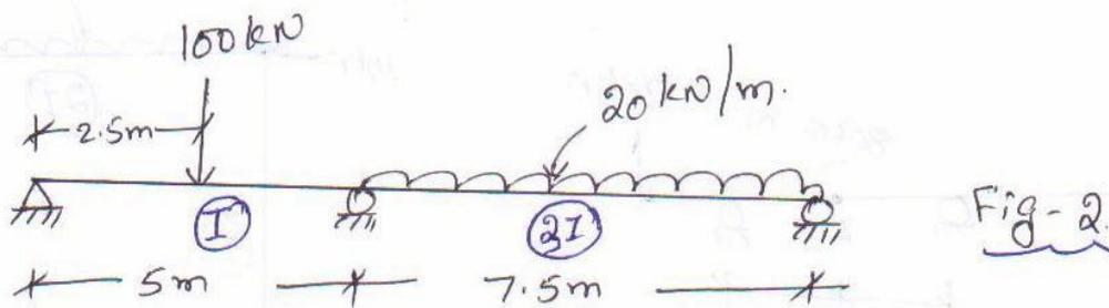
2. Analyse the frame shown in the Fig.2, by moment distribution method. Draw SFD & BMD
