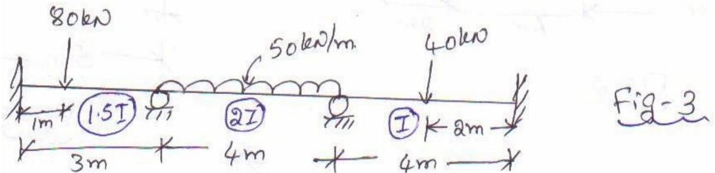
2. Analyse the frame shown in the Fig.3, by Kani's method.
