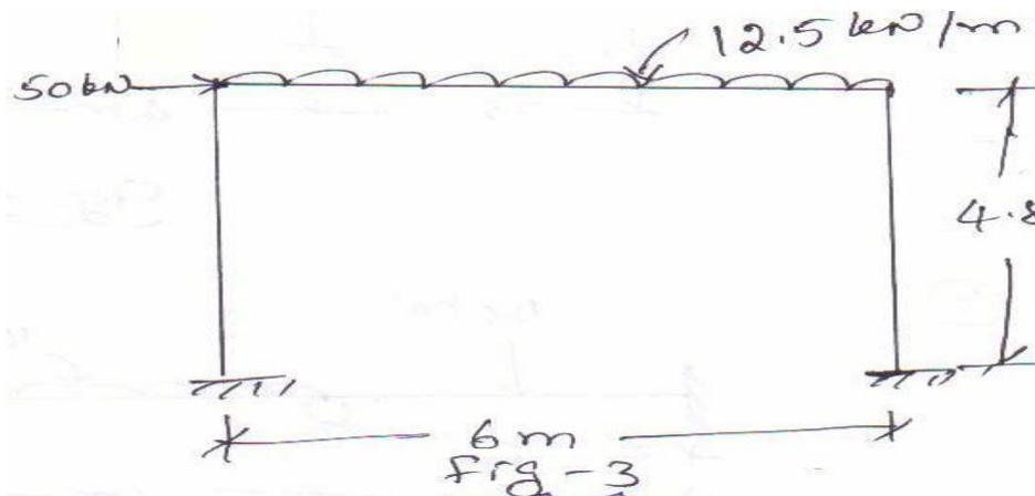
4. Analyse the beam shown in the Fig.3, by Kani's method.
