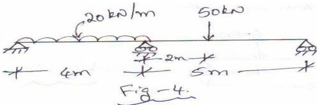
4. Analyse the beam shown in the Fig.4 using flexibility method
