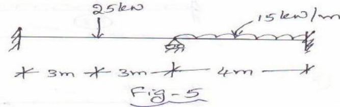
3. Analyse the beam shown in the Fig.5, using stiffness method
