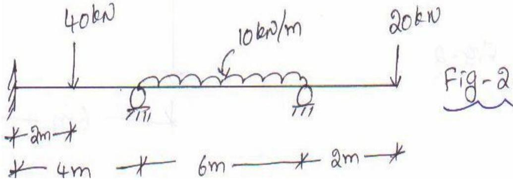
4. Analyse the frame shown in the Fig.2, by moment distribution method. Draw SFD & BMD
