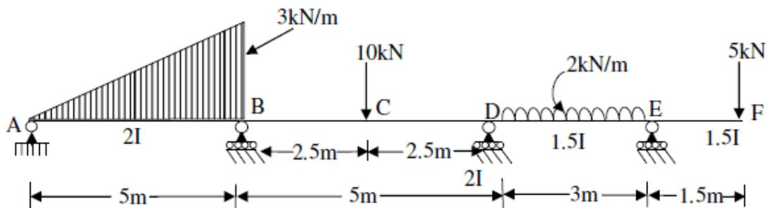
5. Analyze the continuous beam shown in Figure 4, by slope-deflection method
