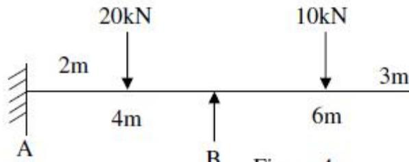
2. Analyze the beam ABCD shown in Figure by Slope-Deflection method and draw bending moment diagram
