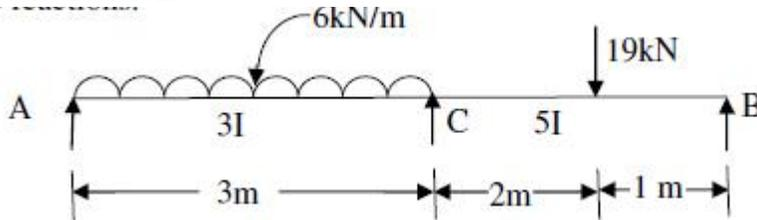
5. A continuous beam has overhangs on both sides as in the Figure 3. Apply three moment equation to determine the support moments. EI is constant throughout.
