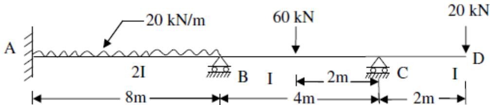
3. A continuous beam ABCD 12 m long is fixed at A and D, and is loaded as shown in Figure 2. Analyze the beam completely if the following moments take place simultaneously i) the end A yields, turning through  $1/250$  radians in a clock-wise direction ii) end B sinks 30 mm in downward direction, iii) end C sinks 20 mm in downward direction. The beam has constant  $I=33.20 \times 10^5 \text{ mm}^4$  and  $E=2 \times 10^5 \text{ N/mm}^2$ . Use slope-deflection method.
