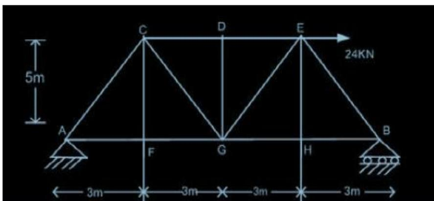
9. Find the forces in the members of truss by method of joints as shown in Figure 1.
