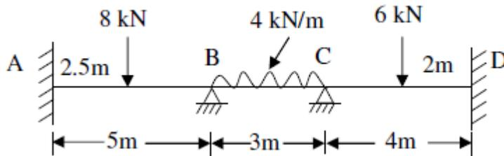
4. Analyze the continuous beam shown in figure, by slope-deflection method.
