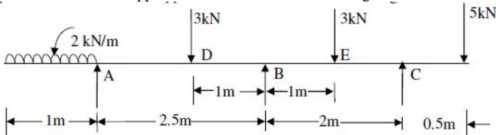
6. Using Clapeyron's theorem, solve the problem of the continuous beam shown in figure 3. EI is constant throughout.
