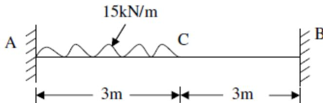
4. Determine the fixed end moments in the beam shown in Figure 2. Support **B** is sinking by 30 mm with respect to support A.
