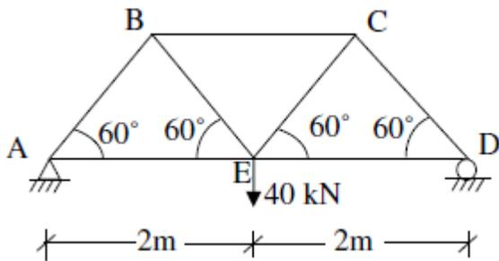
6. Determine the Reaction at A and the moment at B as shown in Figure 3. Use Strain Energy method.
